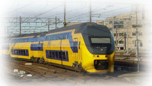
France, Netherlands, Japan, ... 1,5kV / DC
