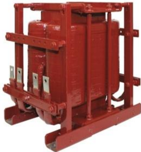
state of the art medium frequency transformer. Example: 110kVA, 8kHz, 44kg
