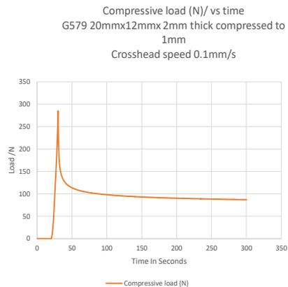
Peak loading at a mere 0.1 [mm/s] or 6 [mm] per minute reaches nearly 300N ( 30kg) between two stainless steel platens. However note how quickly the load drops once the crosshead stops moving and the final loading is about a third of the peak load.
